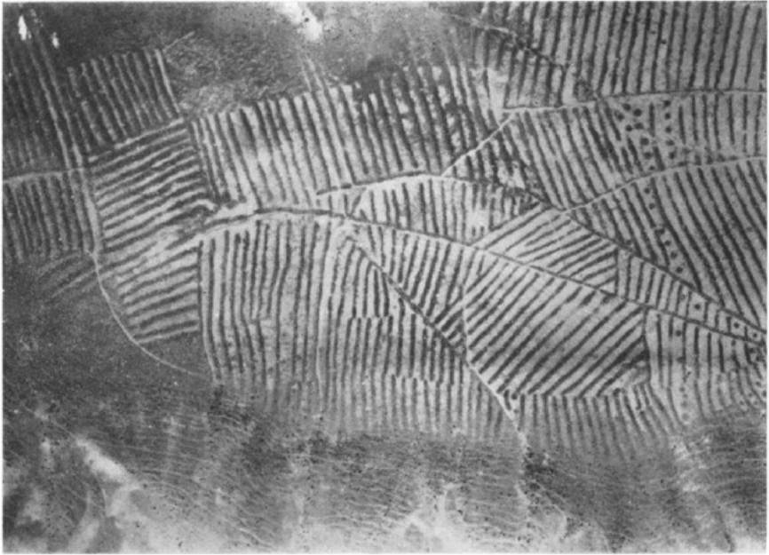
Fig. 11. Qetsiot near Nitsanah. Rows of pebbles, with teleilat el-'anab among them, converging on water channels, designed to help collect runoff of occasional rains and lead it to terraced fields in the Wadi Hafir at bottom of picture. Photo: Israeli Air Force.
