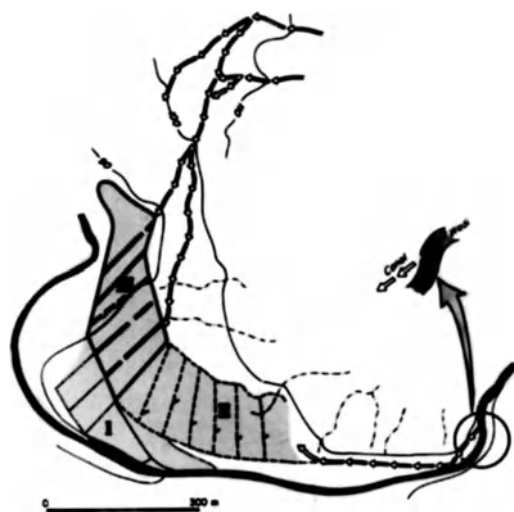
a. Aerial photograph of the diversion system of Kurnub (Photo L. Evenari). b. Field survey of the Kurnub system. Dotted lines Remains of walls of Stage I. Dashed lines Terrace walls of stage II. Solid lines Terrace walls of stage III. Arrows indicate the diversion channel leading water from Wadi Kurnub ( heavy black line ) to the system. Inset Enlargement of diversion dam in Wadi Kurnub
