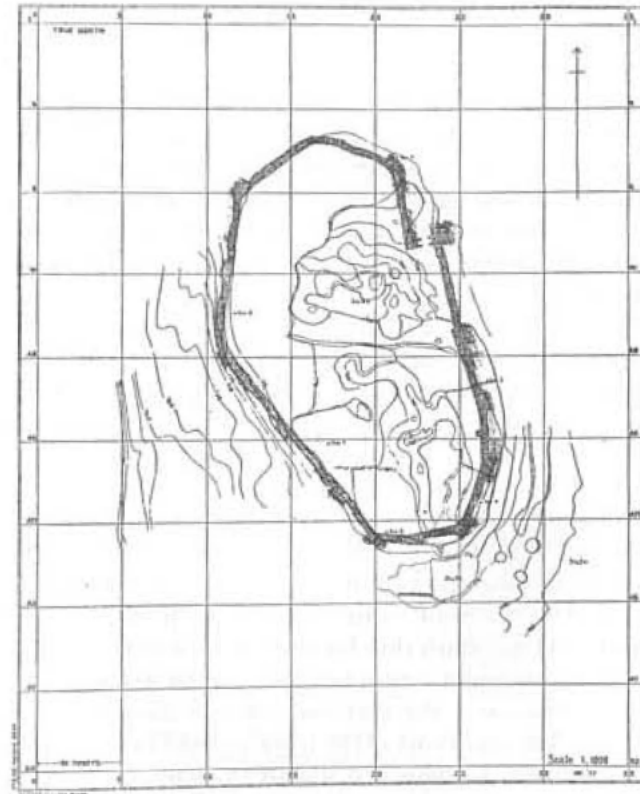
Fig. 1. Asa's fortification wall, completely excavated, laid out on a grid of 50-meter squares. Contours are at 2-meter intervals. Fixed survey stations are indicated. Highest elevation above sea level, 785 meters, or 2575 feet. Scale, 1:1000. P.I. Photo 1182.
