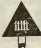
Railway crossing with gate
