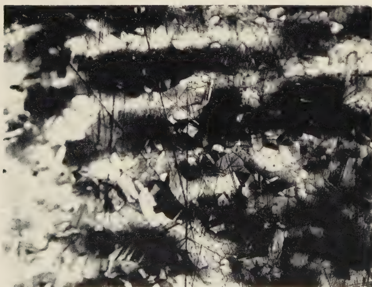
FIG. D. Microstructure of Late Bronze Age dagger (see Fig. C) showing cored and twinned structure of uncorroded bronze. \times 400 diams.
